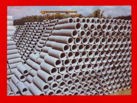
OKA Concrete Porous Pipes are manufactured in accordance with BS 1194-1969 and MS 525-1986. They are manufactured by a combination of high frequency vibration and extrusion method which produces a strong pipe of high and consistent quality and are extensively used for sub-soil drainage to meet a variety of needs.
